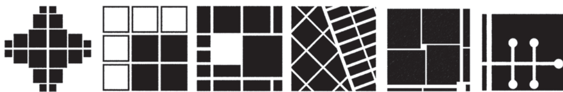
Figure 8. Spatio-formal processes with predictable design outcomes: (left to right) extension, expansion, block subdivision, deformation, marginal separation by linear integration, and discrete separation by linear segregation (Source: Major, 2018; Major et al. , 2023).
