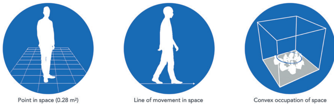
Figure 5. The basics of representation of space used in space syntax research: (left) a point in space using grid elements, such as the average standing area of a human being ( 0.28\text{m}^2 ), (center) a line of movement, and (right) the convex space for human occupation of space where everyone can see and be seen by everyone else (Source: Tannous et al., 2021).
