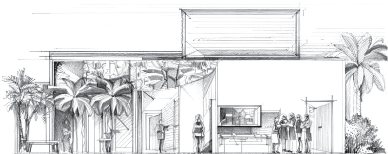
Figure 8. An ideal graphic sketch of a section of the building that illustrates the intersection between the health-care-related areas and the welcoming spaces, inspired by traditional West African architectural models such as open courtyards, impluviums, and verandas. A synthesis of heritage and innovation in healthcare architecture fosters a welcoming, protective environment. Prioritizing sustainability and environmental balance, this design paradigm addresses current and future medical challenges within a global health framework, focusing on comprehensive care for vulnerable populations. The architecture seamlessly integrates with the natural landscape, achieving a zero-impact footprint while effectively serving its healthcare function.
