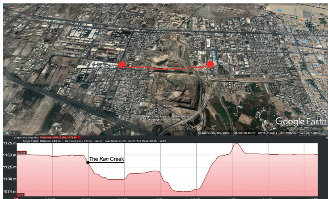
Figure 3. Topographic section of the excavated pits within the study area (Google Earth Pro, 2023).
